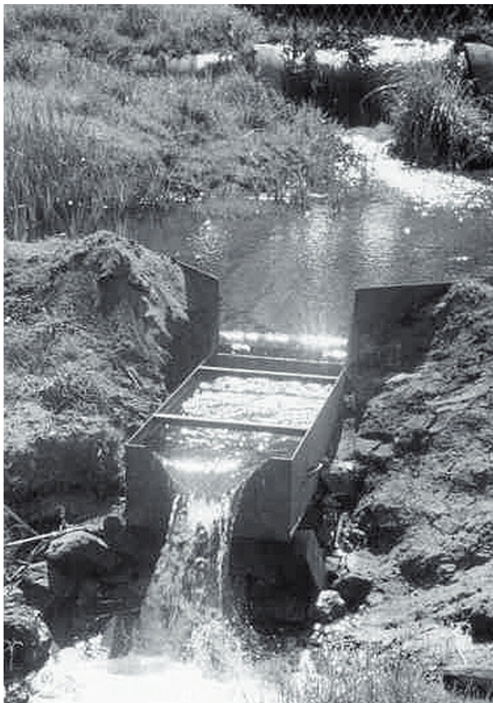
Figure 3.7: A small v-notch weir tank providing flow measurement for clean, treated water leaving a coal processing plant at a South African colliery. (Photo: P. Younger).
