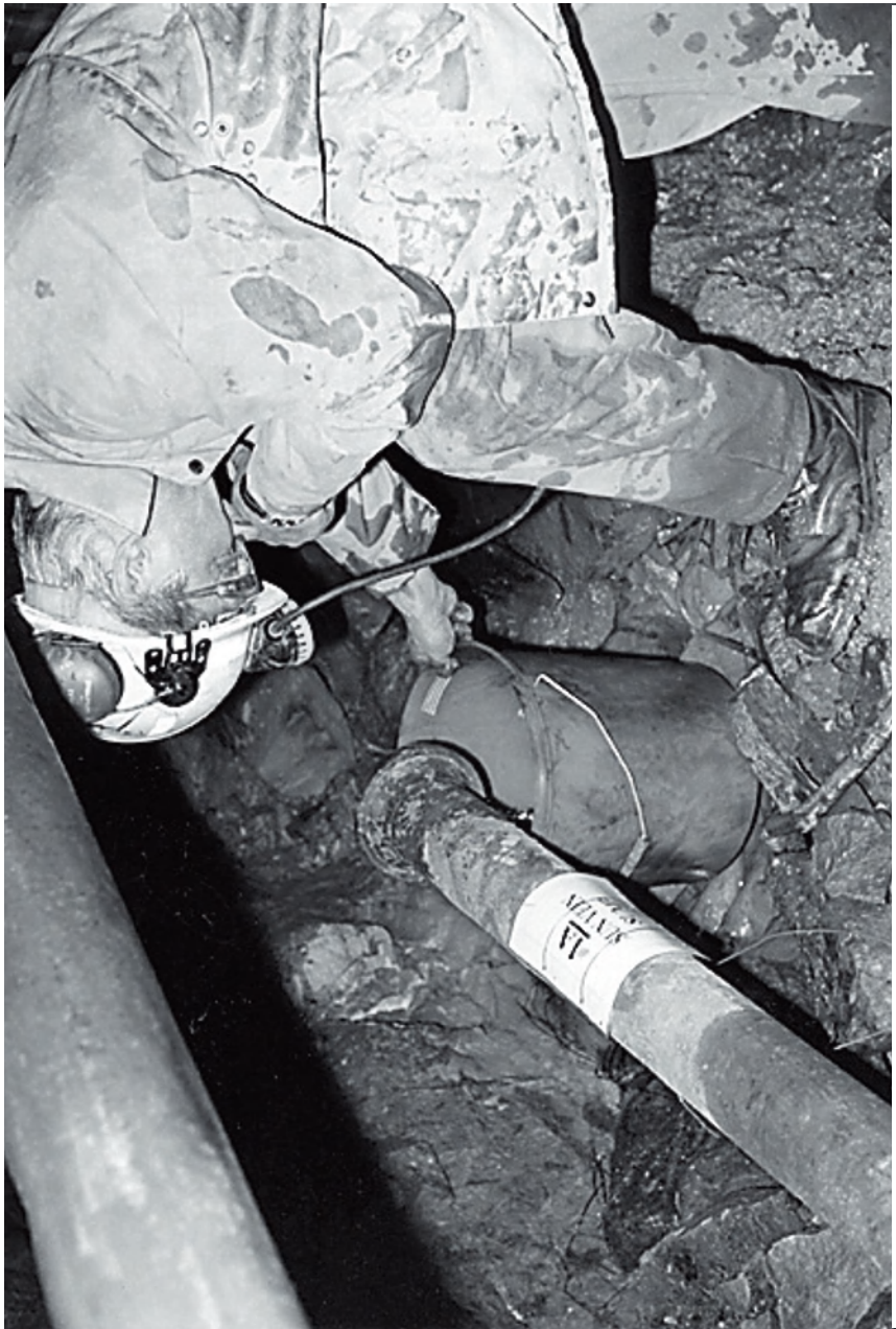
Figure 3.10: Measuring a feeder underground, by diverting it through a pipe whence it is readily measured by bucket-and-stopwatch. John Evans is making the measurements on the Upper Whin Sill Drib, Frazer's Grove Fluorspar Mine, Weardale, UK. (For details of the mine and the use of the data collected, see Younger, 2000b). (Photo: A. Doyle).
