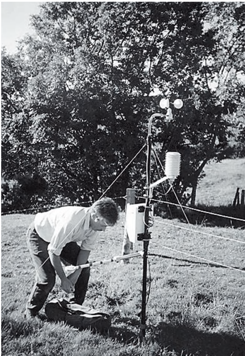
Figure 3.5: A modern, modular automatic weather station (AWS). Incoming radiation is measured by the short mast on the top of the instrument, and net radiation by a transparent sensor in the arm sticking out to the left. Wind speed and direction are measured by the vane and anemometer attached to the top right of the frame. Air temperature and humidity are measured by devices mounted in the louvered white box on the right of the AWS. The other white box (non-louvered) attached centrally to the frame houses the data logger, from which Geoff Parkin is preparing to download data using a portable computer. (Photo: P. Younger).
