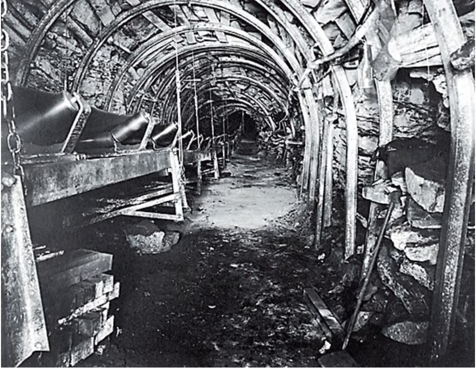
Figure 1.9: District roadway (“main gate”). Closer to the working face than in Figure 1.8, this is a major route by which coal is brought out from the working face to the locomotive haulage roadways, by means of the conveyor belt in the left-hand side of the view. (Photo: A. Doyle).
