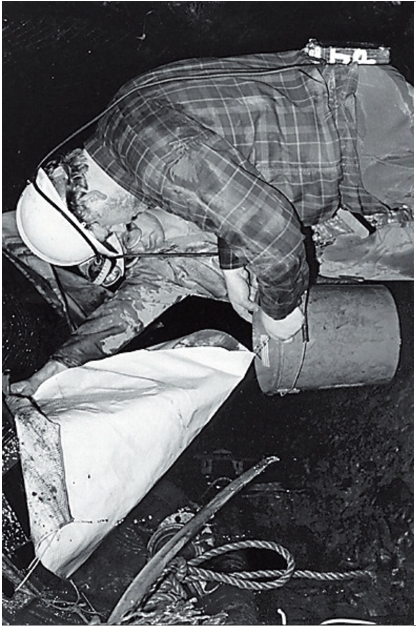
Figure 3.11: Collecting numerous small drippers associated with an old ore hopper using a tarpaulin, facilitating bucket-and-stopwatch measurement. (The tarpaulin is improvised from 'brattice cloth', i.e. canvas normally used for sealing unwanted ventilation routes). John Evans and Paul Younger are making the measurement on the 285E Level of Frazer's Grove Fluorspar Mine, Weardale, UK. (For details of the mine and the use of the data collected, see Younger, 2000b). (Photo: A. Doyle).
